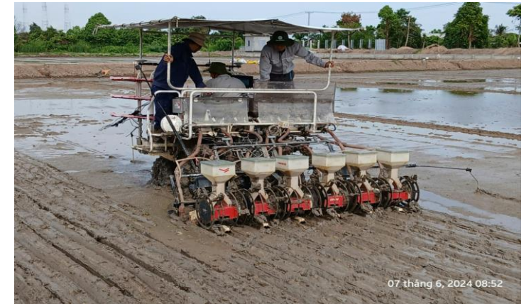
Seeding by Cluster Seeding Machine Incorporated with fertilizer deep placement
