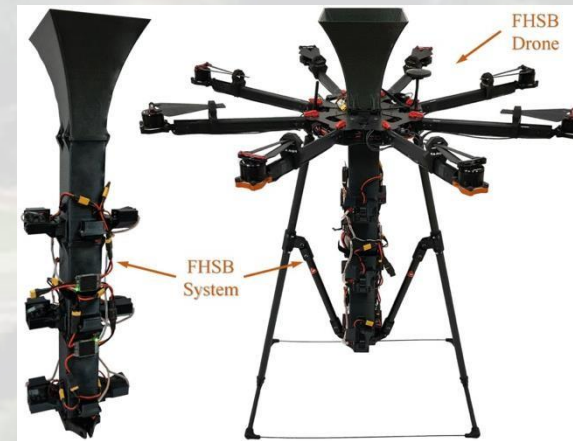
Bulky on-board replacement system
