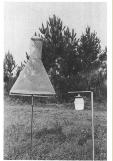
Fig. 1. Hartstack 75-25 cm screenwire cone trap (left) and IP moth trap (right). The IP trap is equipped with a Vapona insecticide strip as a killing agent.
